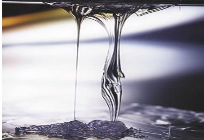
Low viscosity liquid silicone rubbers.
